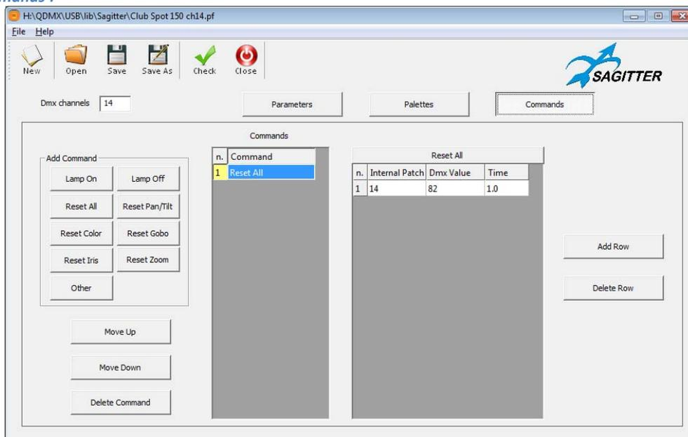
After the data editing, has been completed, it's possible to make a quick check using the 'Check' button, in order to spot any big error in the DMX channel. If the 'Check' result is positive, you can proceed to save the fixture in the proprietary format of the QUIVER console, which is a file type '**.pf**'. At this point, we recommend to test the new fixture file the with some cue from the console, before using it in a show.
