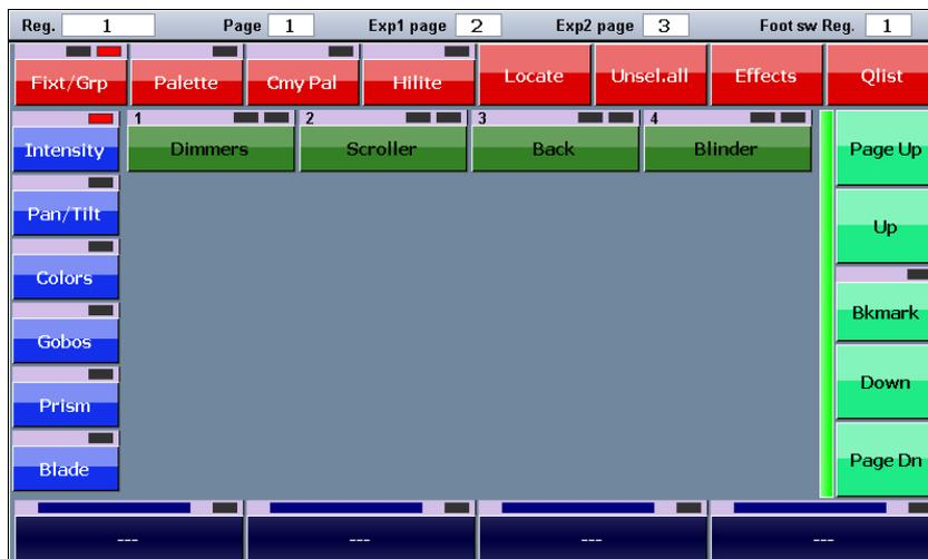
The fixture can be selected one by one using of the correspondent buttons or together using the ‘Group’ way: you can switch alternately from the fixture view to the group view using the Fixture/Group button. Pressing the ‘Intensity’, ‘Pan Tilt’, ‘Colors’, ‘Gobos’, ‘Prism’ and ‘Blade’ buttons the parameters of the selected fixtures are assigned to the 4 Touch Sliders.
