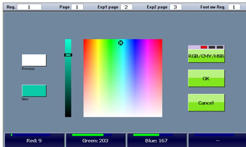
Colors can be selected directly from the color bitmap and luminosity slider on the display or using the first three Touch Slider. The RGB/CMY/HSB button selects the input mode scrolling through the three available color modes (Red / Green / Blue, Cyan / Magenta / Yellow and Hue / Saturation / Brightness).
