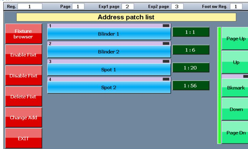
Pressing the 'Fixture browser' button you can access the library (that can be located whether in the SD internal memory or in the USB memory) and add the fixtures desired to the patch of the show.
