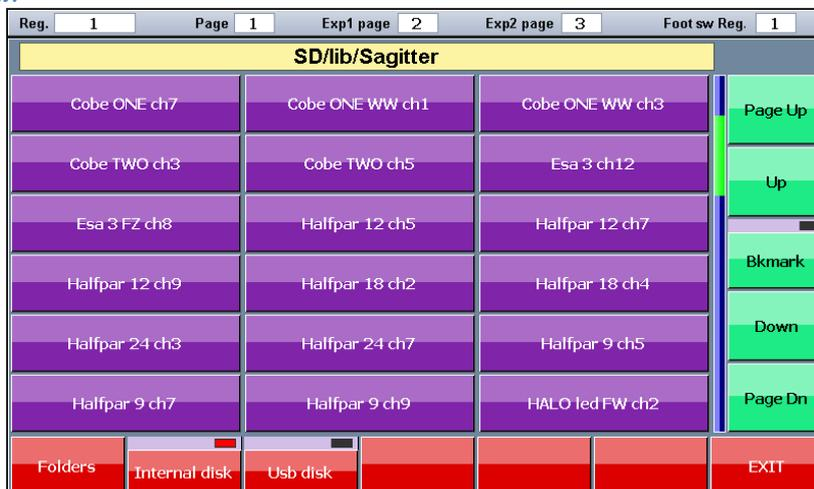
Pressing the button of the desired fixture the "Add fixture" window appears, that allows to set up the number of fixtures of the selected type to be added at the show.
