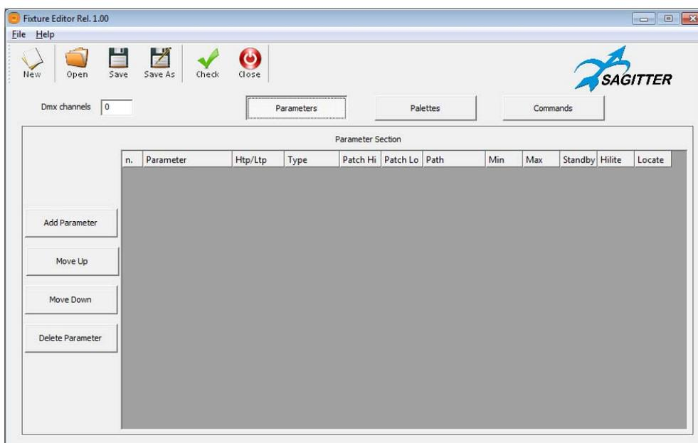
Using the commands 'Add Parameter', 'Move Up', 'Move Down', 'Delete Parameter' you can edit the parameters, taking them from the user manual of the fixture to be created.
