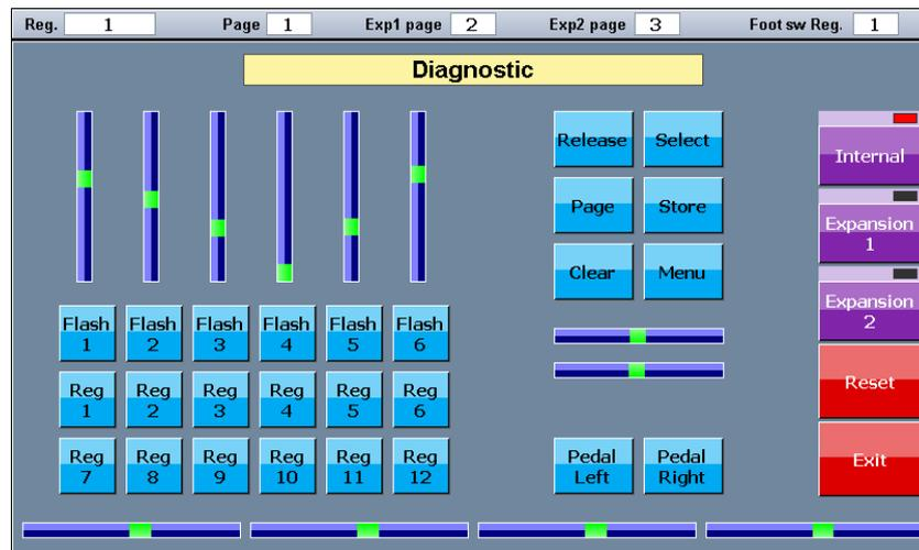
When any console's command is activated (keys, slider potentiometers, Touch Slider, joystick), the action is shown on the screen, allowing to check whether the command is working properly.
