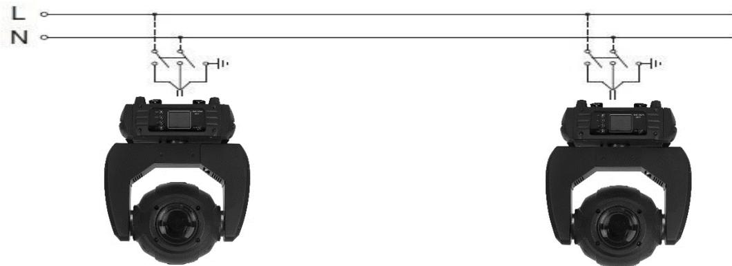
The device must be connected to a power supply system with a proper earth system. Moreover, it is recommended to protect power supply lines of the products from indirect contact and / or shorting to earth by using appropriately sized anti electrical shock switch. The electrical connection must be carried out by a qualified electrician. Ensure that the mains frequency and voltage correspond to those for which the device is designed, as shown in the electrical data label.
