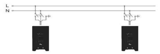
The device must be connected to a power supply system with a proper earth system. Moreover, it is recommended to protect power supply lines of the products from indirect contact and / or shorting to earth by using appropriately sized anti electrical shock switch.
