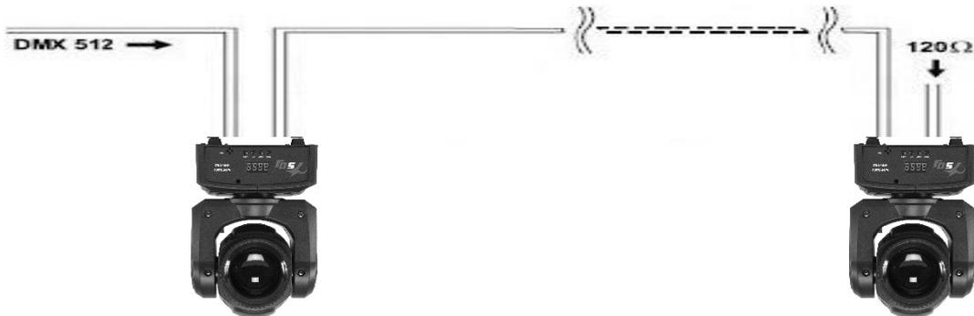
Use a cable conforming to specifications EIA RS-485: pole twisted, shielded, 120Ohm characteristic impedance and low capacity (SAGITTER SG DMX3 – SG DMX5).
