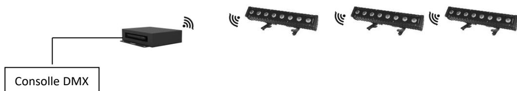
To connect the transmitter to a DMX console use a cable conforming to specifications EIA RS-485: pole twisted, shielded, 120Ohm characteristic impedance and low capacity (SAGITTER SG DMX3 – SG DMX5).
