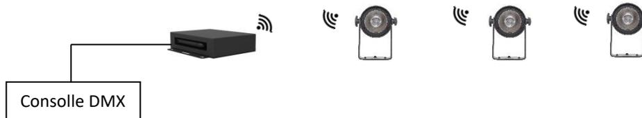
To connect the transmitter to a DMX console, use a cable conforming to specifications EIA RS-485: pole twisted, shielded, 120Ohm characteristic impedance and low capacity (SAGITTER SG DMX3 – SG DMX5).
