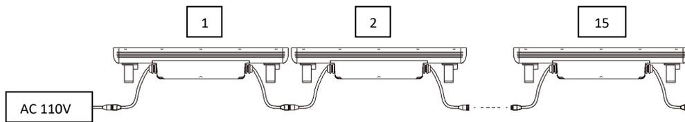
The device must be connected to a power supply system with a proper earth system. Moreover, it is recommended to protect power supply lines of the products from indirect contact and / or shorting to earth by using appropriately sized anti electrical shock switch. The electrical connection must be carried out by a qualified electrician. Ensure that the mains frequency and voltage correspond to those for which the device is designed, as shown in the electrical data label.
